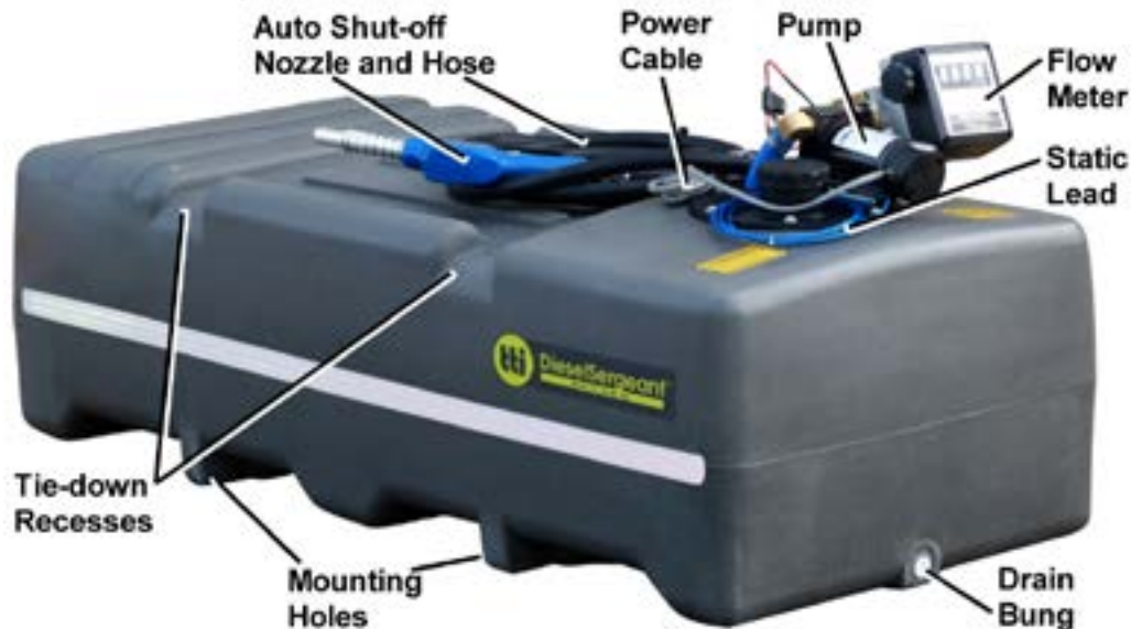
Figure 1 - Component Identification - 1,000 L DieselMajor
