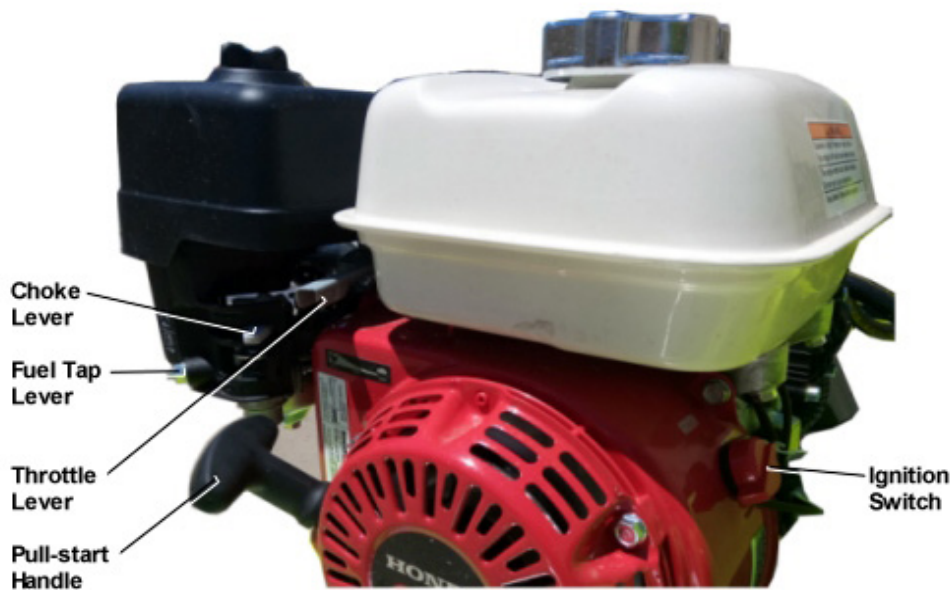
Figure 6 – Petrol Pump Details
