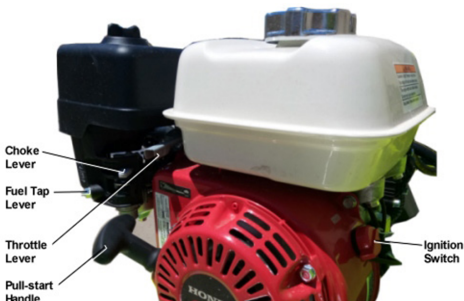
Figure 2 –Honda Pump Engine Details
