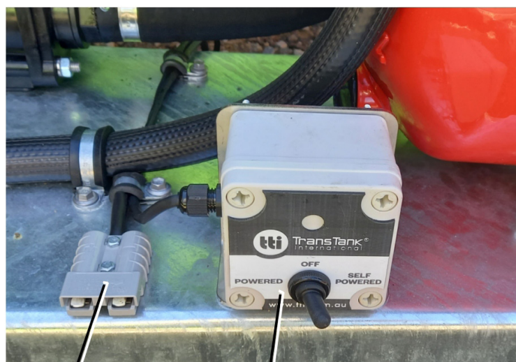
Anderson Plug Solenoid Control Switch
