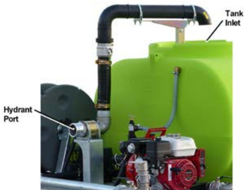
Figure 6 – Hydrant Filling Operation (optional fill kit)
