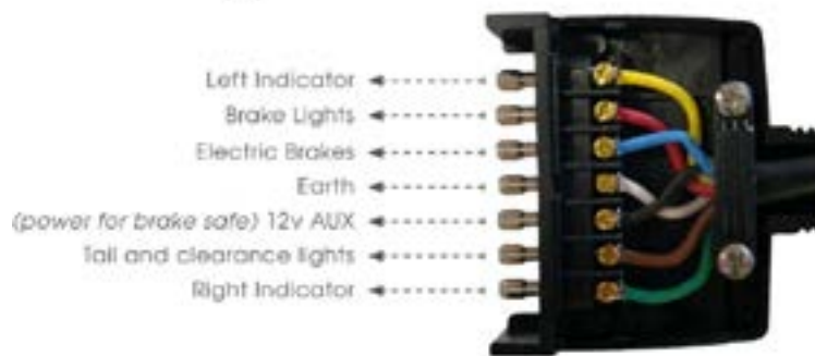
7-Pin Plug Wiring Requirements
