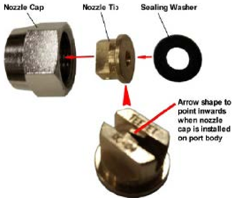
Figure 6 – Off-centre end jet nozzle installation
