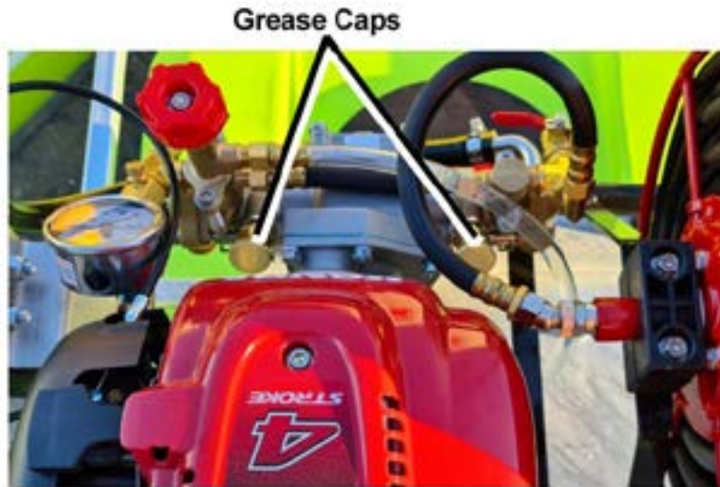
Figure 11 – Grease Caps Maintenance
