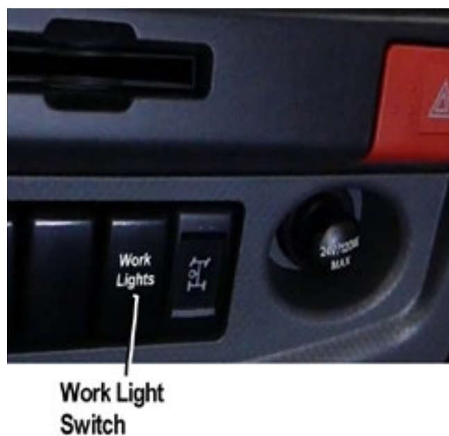
Figure 12 – Work Lights Switch
