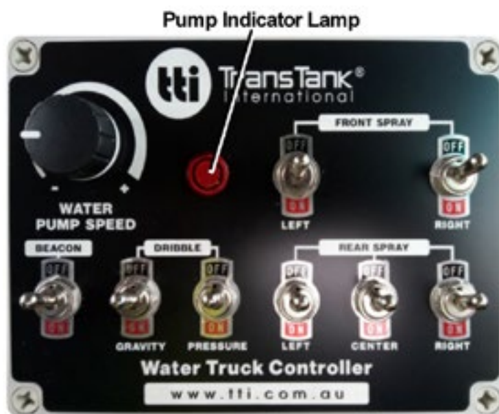
Figure 3 – In-cab Control Panel – Hydraulic Pump Unit
