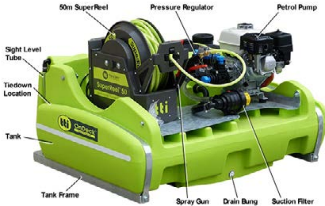
Figure 2 – Component Identification – Standard Edition with Petrol Pump & 50m SuperReel
