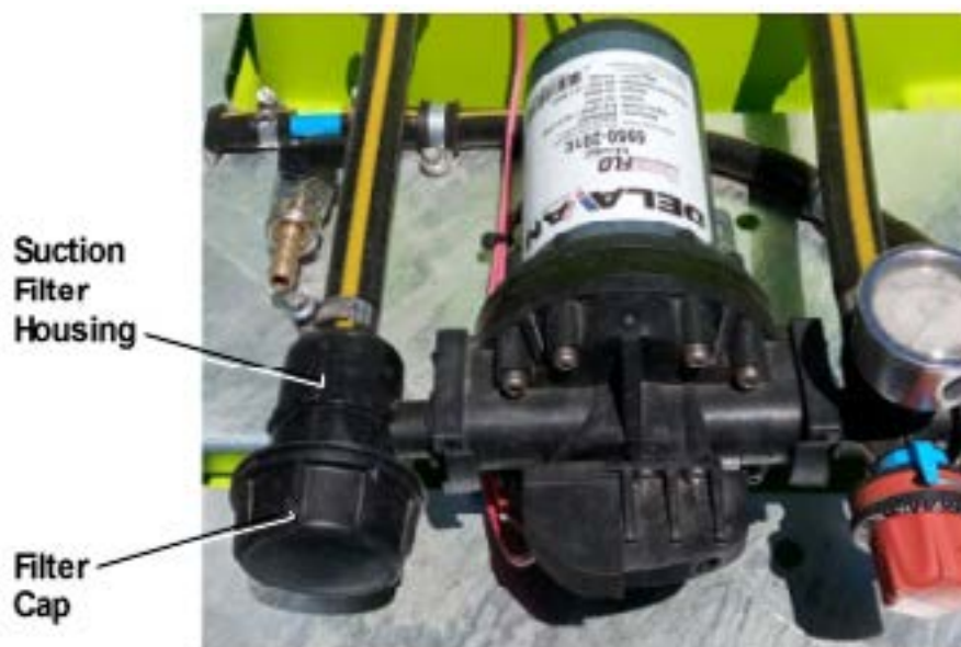
Figure 16 – Electric Pump's Suction Filter
