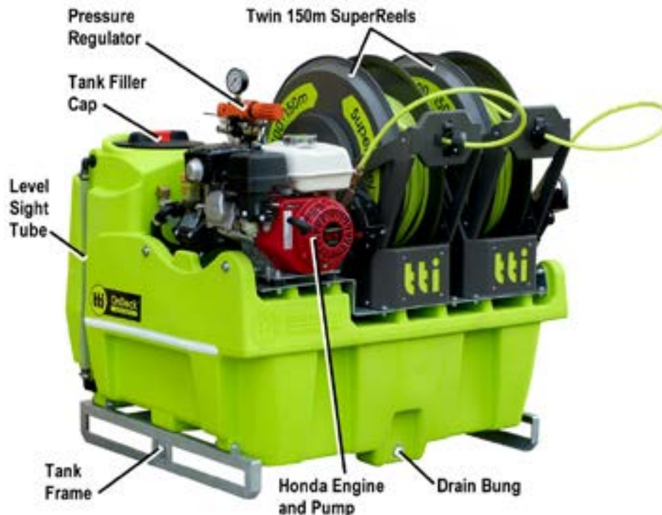
Figure 4 – Component Identification – Compact Edition with Petrol Pump & Twin 150m SuperReels
