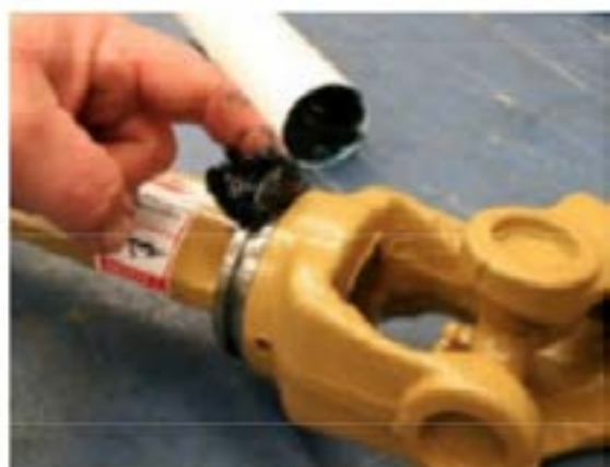
Cut Drive Tubes, Remove Burrs, Grease and Reassemble
