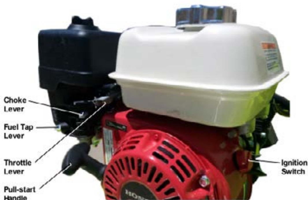
Figure 4 – Petrol Pump Details
