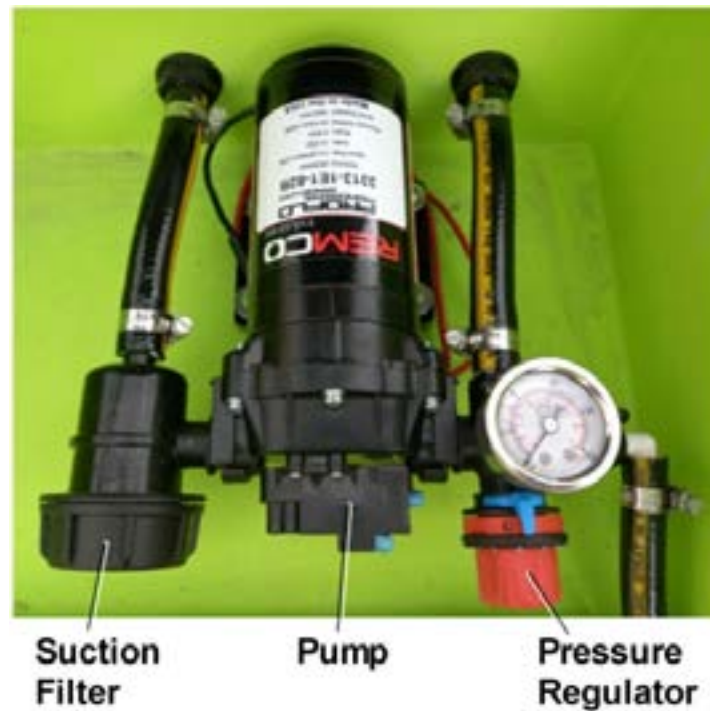
Figure 11 – Electric Pump's Suction Filter
