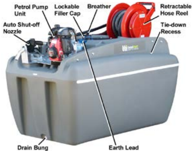
Figure 1 - Component Identification - 1,000 L DieselMajor
