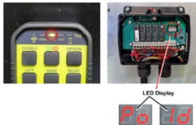
Figure 18 – Remote Control Unit and Transmitter Indication
