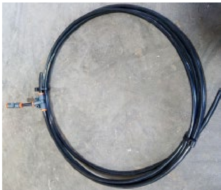
Figure 2 – Pneumatic Hose and Tee Piece
