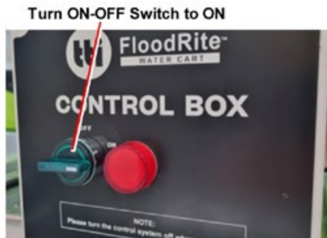
Figure 19 – Control Box ON-OFF Switch to OFF
