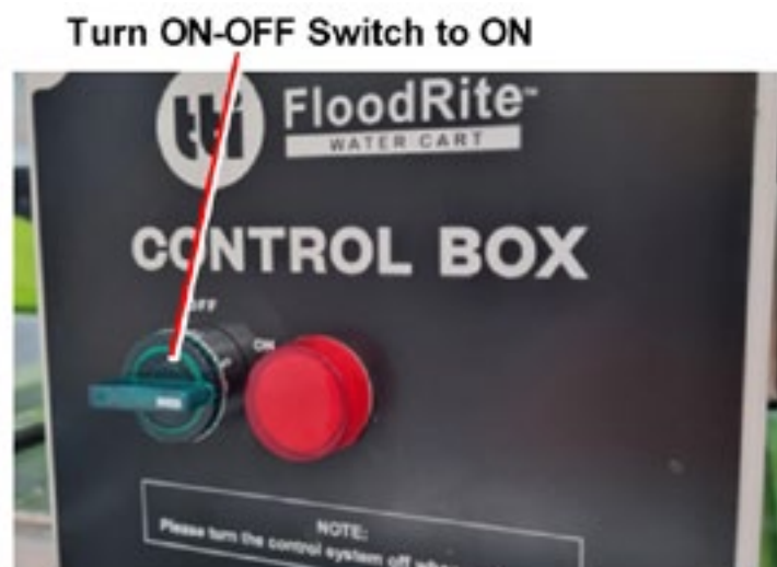
Figure 17 – Control Box ON-OFF Switch to ON
