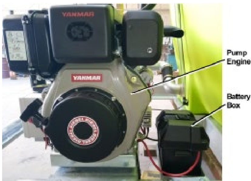
Figure 3 – Pump Engine and Battery (Diesel unit shown)
