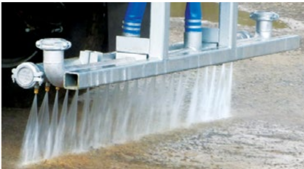
Figure 10 – Dribble Bar (Typical)
