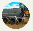
65mm 2T-rated Galvanised Axles with 15" Landcruiser Wheels
